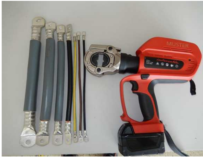
AP60-2: Battery operated hydraulic crimping tool 60kN up to 300mm 2
