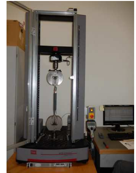
pull compression machine up to 50kN
