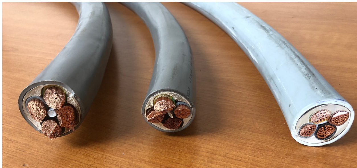
cables that were tested: 4x95(klasse5), 4x70(klasse5) Vultflex and an 4x70(klasse2) Hultflex
