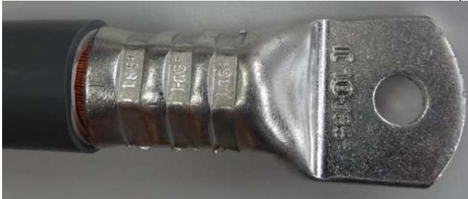
NEXANS cable 185mm 2 with ICR18510 and MI185-CK (3 crimps with AP60-2)
