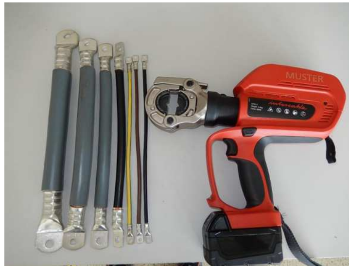
AP60-2: Battery operated hydraulic crimping tool 60kN up to 300mm 2 pull compression machine up to 50 kN
