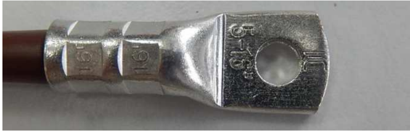
NEXANS cable 16mm 2 with ICR165 and MI16-CK (2 crimps with AP60-2)
