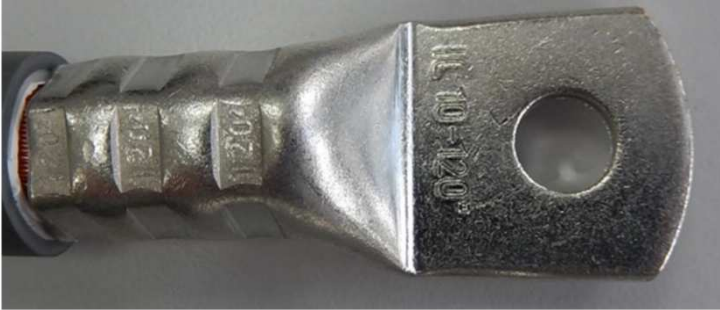
NEXANS cable 120mm 2 with ICR12010 and MI120-CK (3 crimps with AP60-2)
