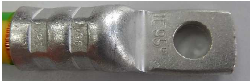
NEXANS cable 95mm 2 with ICR9510 and MI95-CK (2 crimps with AP60-2)
